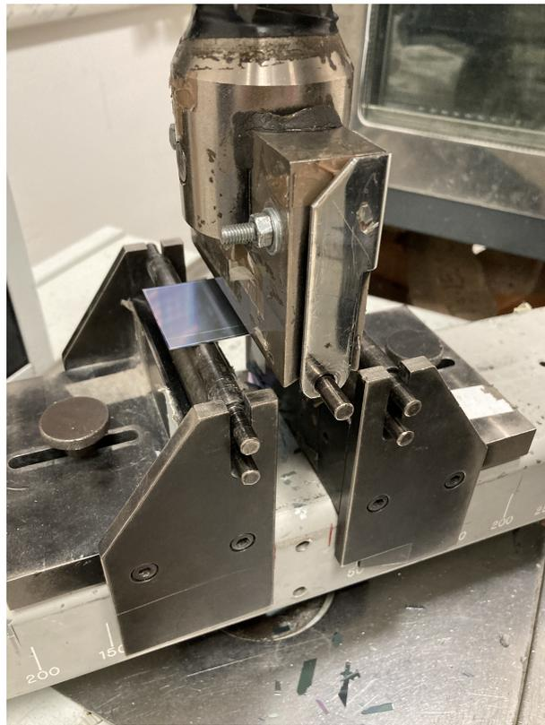
Figure 6. Three-point bending test setup.
