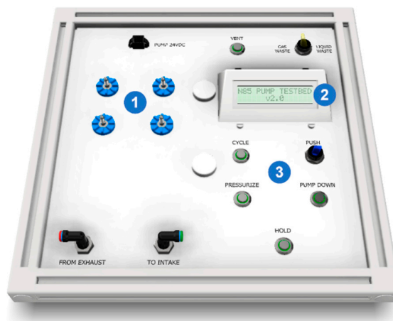
Figure 2: (1) captive panel screws and rubber vibration dampening grommets; (2) LCD mounted on the bezel; and (3) illuminated controls.
