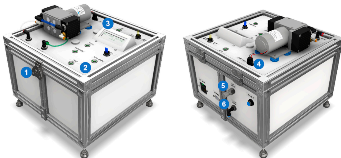
Figure 1: (1) quick-turn draw latch, (2) control panel, and (3) custom LCD bezel, (4) power plug for the pump, (5) muffler for the gas exhaust, (6) and elbow fitting pointing downwards to drain exhaust liquids.
