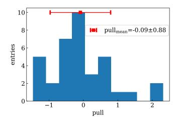
**Figure 13.** Histogrammed pull for calibrated energy deposition in silicon. The mean of the distribution and the corresponding standard deviation are highlighted in red.
