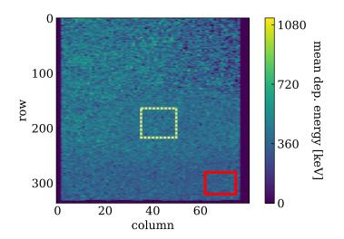
**Figure 4.** Map of mean deposited energy for every pixel measured with a beam energy of  $E_{\text{phantom}} \approx 65.4$  MeV. The colored frames indicate two example regions of interest, highlighting the variation of the deposited energy across the regions of the staircase phantom.
