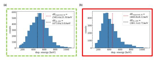
**Figure 7.** Deposited energy spectra for (**a**) phantom thickness of 2.0 cm, corresponding to  $E_{\text{sensor}} \approx 36.8 \text{ MeV}$  and for (**b**) phantom thickness of 1.2 cm, corresponding to  $E_{\text{sensor}} \approx 49.8 \text{ MeV}$ . The frames identify the ROIs according to Figure 4.
