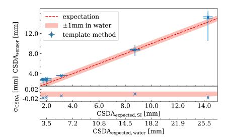
**Figure 16.** Comparison of  $CSDA_{expected, SI}$  for different initial beam energies and the corresponding measured CSDA range  $CSDA_{sensor, est}$  estimated by using the template. The red dotted line indicates the expectation and the light red colored interval the deviation  $\pm 1 \text{ mm}$  of  $CSDA_{expected, water}$ . The accuracy of the estimator is illustrated using the parameter  $\sigma_{CSDA}$ .
