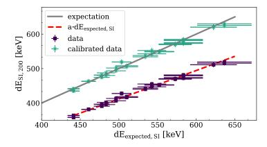
**Figure 9.** Measured mean deposited energy in silicon  $dE_{SI,200}$  versus the expected deposited energy  $dE_{expected,SI}$ . Results are plotted before (purple squares) and after calibration (green stars).
