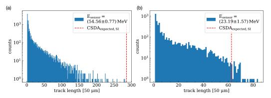
**Figure 10.** Track length distributions along the beam axis for all tracks measured for two different energies: (a)  $E_{\text{sensor}} = (54.56 \pm 0.77)$  MeV and for (b)  $E_{\text{sensor}} = (23.19 \pm 1.57)$  MeV. The dotted red line indicates the expected CSDA range of the protons in the silicon sensor.
