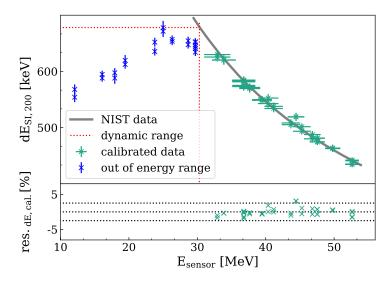
**Figure 12.** Calibrated results of the mean deposited energy  $dE_{SI,200,cal}$  and their relative deviation from the NIST expectation. The minimum energy  $E_{sensor, min} = 30.4 \text{ MeV}$  measurable with this configuration of the detector and the resulting data, which had to be excluded from the analysis, are highlighted.
