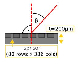
**Figure 1.** Sketch to define the incident angle  $\beta$  with respect to the normal of the detector surface. The thickness *t* of the sensor and the pixelation are indicated.
