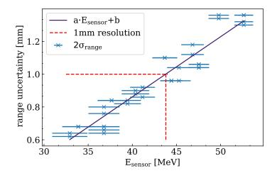
**Figure 14.** Uncertainty of the measured proton range in water as a function of the expected incident proton energy  $E_{\text{sensor}}$  ( $a = (0.037 \pm 0.002) \frac{\text{mm}}{\text{MeV}}$ ,  $b = (-0.60 \pm 0.08)$  mm). The upper energy limit  $E_{\text{max.}} = (43.8 \pm 3.2)$  MeV to fulfill the QA requirement is highlighted.
