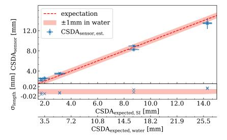
**Figure 15.** Comparison of  $CSDA_{expected, SI}$  for different initial beam energies and the corresponding measured CSDA range  $CSDA_{sensor, est}$  estimated by using the longest measured cluster length. The red dotted line indicates the expectation and the light red colored interval the deviation  $\pm 1$  mm of  $CSDA_{expected, water}$ . The accuracy of the estimator is illustrated using the parameter  $\sigma_{length}$ .
