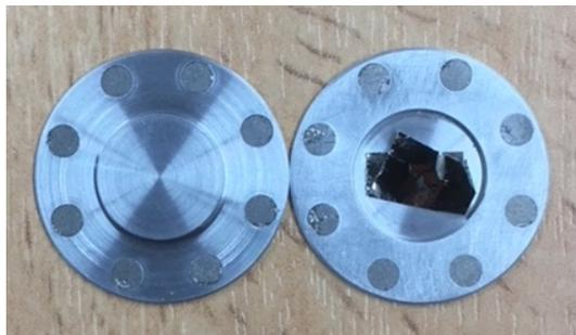
**Figure 2.** The two halves of the “coin” target held together by eight couples of permanent magnets. The rear half (on the left) is water cooled and matches the front half (on the right) that is used to degrade the beam to the desired energy.
