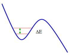
**Figure 2.** Profile of potential energy  $U(\phi) = -E_J \{\cos \phi + i_b \phi\}$  of the Josephson phase qubit.
