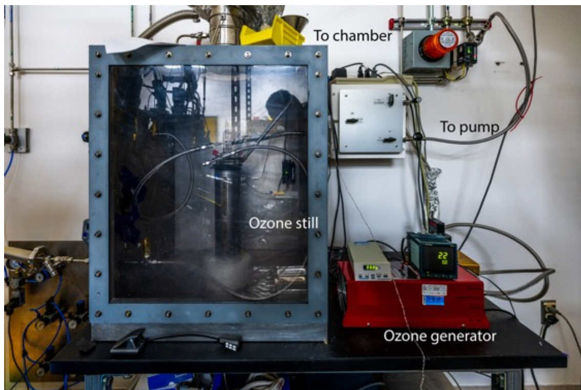
Figure 4. Photo of the ozone distillation system. A commercial arc-discharge ozone generator generates an ozone and oxygen gas mixture from a pure oxygen gas supply. The mixture is cooled in a quartz vessel (ozone still) with liquid nitrogen as a coolant. Then, the mixture is warmed up so that O_2 evaporates and is pumped out, leaving a pure O_3 liquid in the still. Ozone vapor is then supplied to the MBE growth chamber when needed. A PID-controlled heater controls the ozone vapor pressure.
