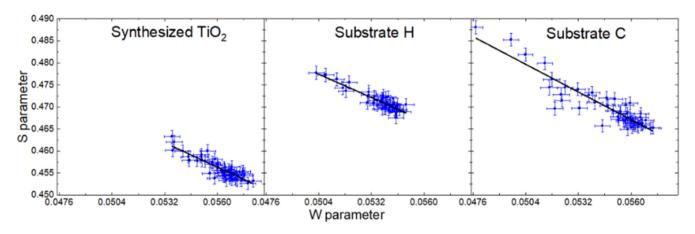
**Figure 10.** S-W plot for synthesized TiO<sub>2</sub>, H, and C substrates. Continuous line represents the average slope.
