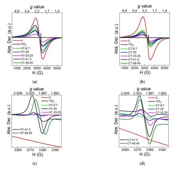
**Figure 6.** ESR spectra between 500 and 5500 G for (a) HT composites; (b) CT composites. ESR spectra around 3375 G for (c) HT composites; (d) CT composites.
