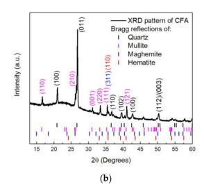
**Figure 1.** (a) SEM image of CFA, (b) XRD pattern for CFA indexed with quartz, mullite, maghemite, and hematite.
