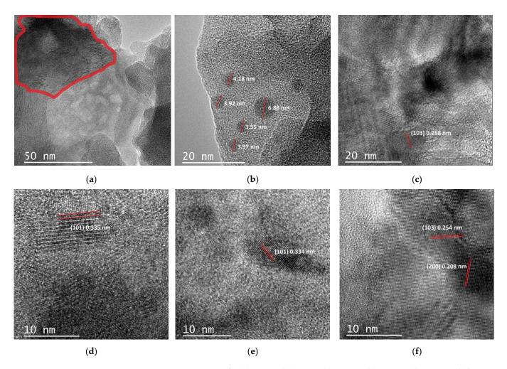
Figure 7. HRTEM images for (a) HT-8.7, (b) HT-25, (c) HT-41.3, (d) CT-8.7, (e) CT-25, and (f) CT-41.3. Red line represents the interface between zeolite and TiO2 in Figure 7a and the lattice spacings for Figure 7b–f.
