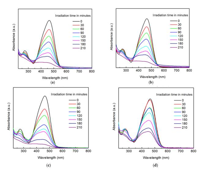
**Figure 13.** UV-Vis spectra of MO solution photoreduction by (a) HT-8.7, (b) HT-25, (c) synthesized, and (d) commercial  $\text{TiO}_2$ .
