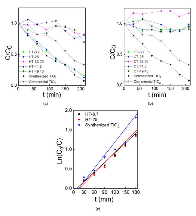
**Figure 14.** Time-dependent degradation of MO by photocatalytic activity of (a) HT and (b) CT composites. (c) The  $ln(C_0/C)$  vs. t plot.
