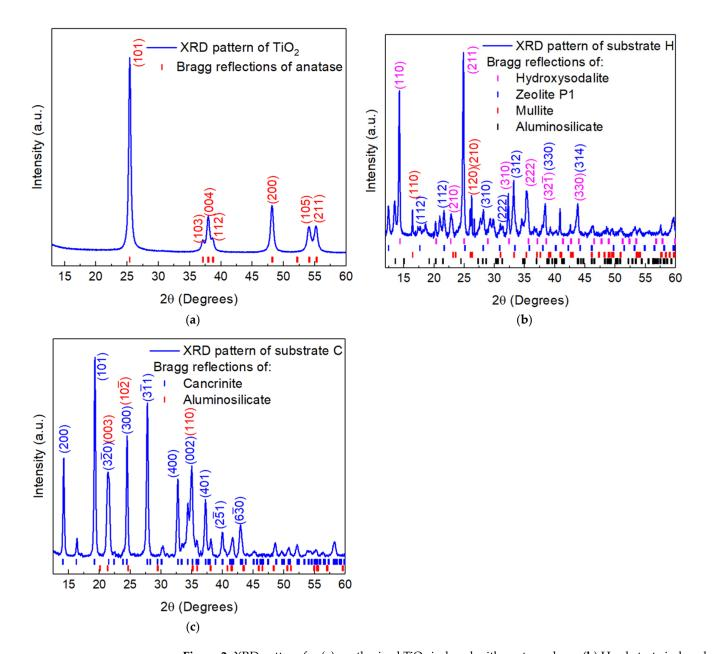
**Figure 2.** XRD pattern for (**a**) synthesized TiO<sub>2</sub> indexed with anatase phase, (**b**) H substrate indexed with hydroxysodalite, zeolite P1, mullite, and sodium aluminosilicate, (**c**) C substrate indexed with cancrinite and an aluminosilicate.
