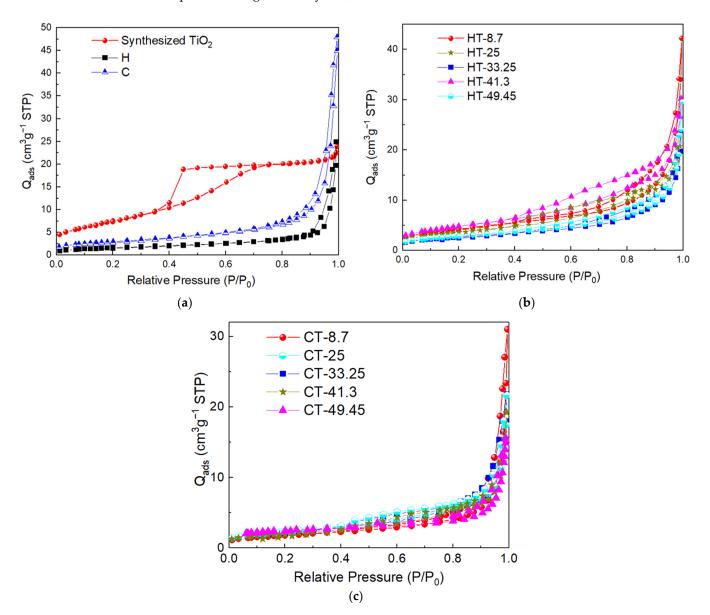
$\textbf{Figure 8.} \ \ \text{N}_2 \ \text{adsorption isotherm of (a) synthesized TiO}_2 \ \text{substrates; (b) HT composites; (c) CT composites.}$
