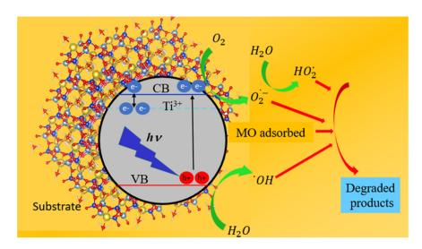
Figure 15. Scheme of photocatalytic mechanism for MO degradation.
