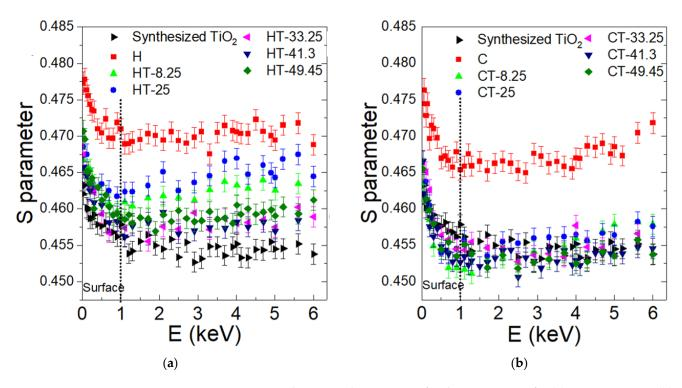
**Figure 9.** Variation with positron beam energy for the S parameter for (a) HT composites; (b) CT composites. Dashed line separates the surface and bulk region.
