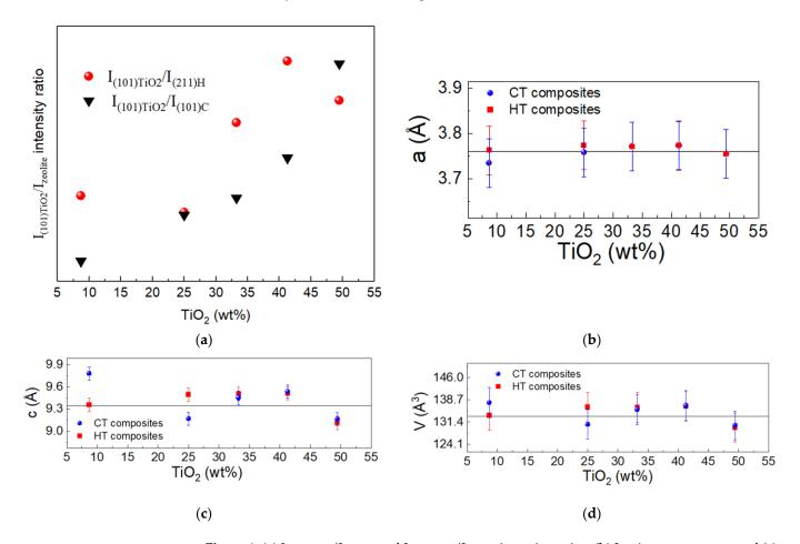
**Figure 4.** (a)  $I_{(101)TiO2}/I_{(211)H}$  and  $I_{(101)TiO2}/I_{(101)C}$  intensity ratios. (b) Lattice parameters a and (c) c; and (d) cell volume. The continuous line represents the value for synthesized  $TiO_2$ .
