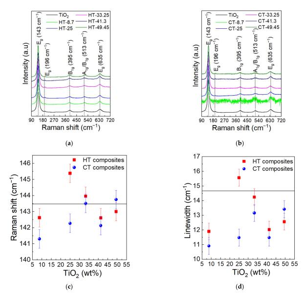
**Figure 5.** Raman shift spectra for (a) HT composites, (b) CT composites, (c) variation of Raman shift, (d) linewidth for the 144 cm<sup>-1</sup> peak as a function of TiO<sub>2</sub> weight percentage. the continuous line represents the parameters for synthesized TiO<sub>2</sub>.
