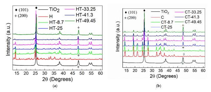
**Figure 3.** XRD pattern for (a) HT composites (b) CT composites. For comparative purposes, the XRD of C, H, and synthesized TiO<sub>2</sub> are depicted.
