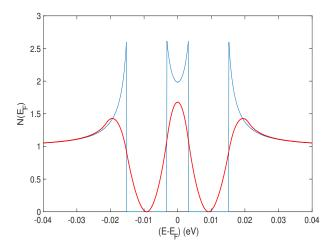
**Figure 3.** A model of how a constant DOS might be deformed when two phonons, one with *k* smaller than and one larger than  $k_F$  are present (thin blue line). Disorder can come from ZPM, thermal vibrations or spin-fluctuations, and has a smearing effect on the DOS with a large increase in  $N(E_F)$  (bold red line).
