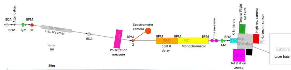
**Figure 8.** Layout of the ARIA beamline. BDA, beam defining aperture; BPM, beam position monitors; I<sub>0</sub>M, intensity meters; M, steering mirror; G, diffraction grating.
