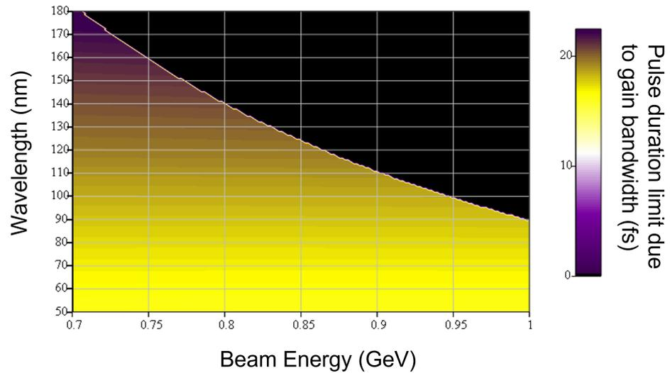
**Figure 5.** Expected photon pulse duration as a function of the electron beam energy (x) and wavelength (y). A 15 fs electron bunch and circular polarization are assumed.
