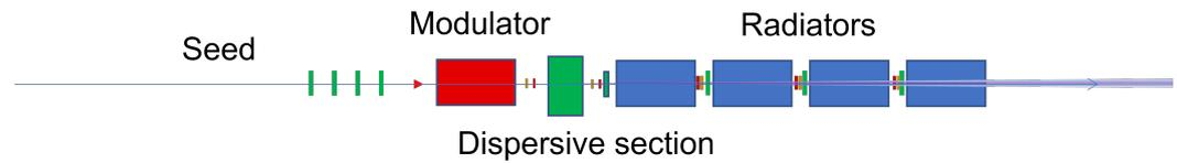
**Figure 2.** Layout of the ARIA HGHG FEL. The seed pulse is superimposed on the electron bunches at the modulator entrance, and the dispersive section is a four-dipole chicane that converts the energy modulation into a density modulation. Its length  $\sim 2$  m is kept constant and the dispersion strength is tuned by varying the dipole magnetic fields. The amplification stage is made up of four radiators.
