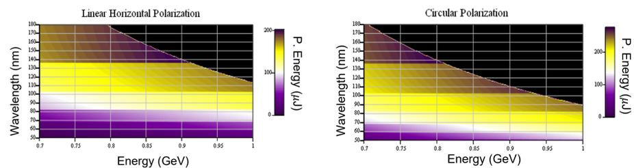
**Figure 4.** Expected photon pulse energy in the long pulse mode as a function of the electron beam energy (x) and wavelength (y). (Left): linear polarization. (Right): circular polarization.
