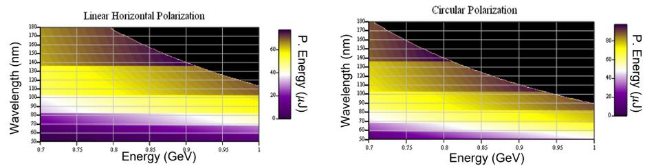
**Figure 3.** Expected photon pulse energy in the short pulse mode as a function of the electron beam energy (x) and wavelength (y). (Left): linear polarization. (Right): circular polarization.
