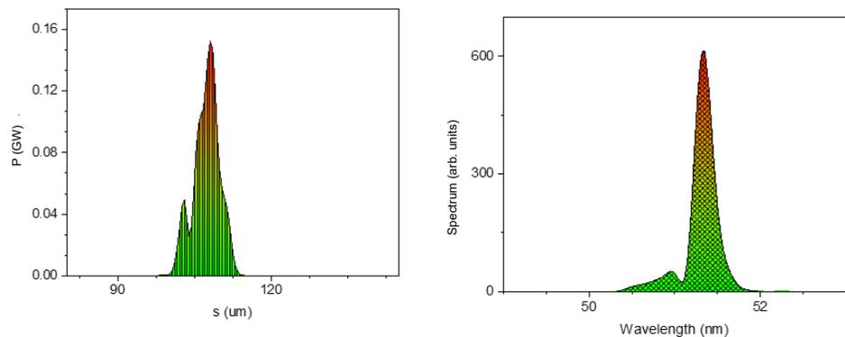
**Figure 7.** FEL emission at 51 nm, ninth harmonic of the 460 nm seed. **(Left):** pulse longitudinal power profile (GW) vs.  $s(\mu\text{m})$ . **(Right):** spectral amplitude (arb. units) vs.  $\lambda(\text{nm})$ . Extraction after four radiators.
