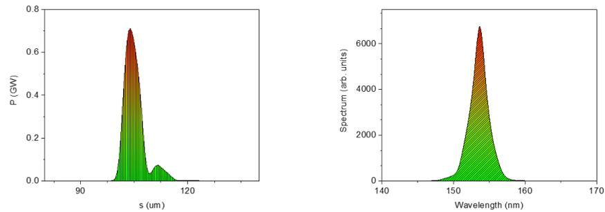
**Figure 6.** FEL emission at 153 nm, third harmonic of the 460 nm seed. **(Left):** pulse longitudinal power profile (GW) vs.  $s(\mu\text{m})$ . **(Right):** spectral amplitude (arb. units) vs.  $\lambda(\text{nm})$ . Extraction is performed after three radiators.
