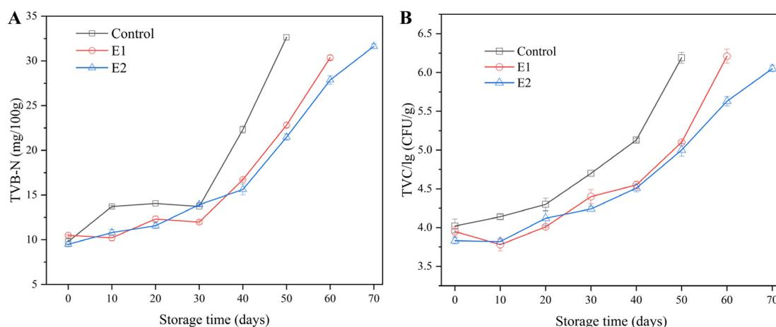
**Figure 4.** TVB-N (A) and TVC (B) of the control shrimp, shrimp preserved in 4% NaCl (E1) solution, and shrimp preserved in 4% NaCl, 0.34% citric acid, 4.23% trehalose, and 0.04% VC solution (E2) during chilled storage.
