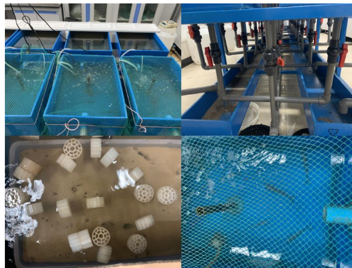
Figure 1. Basic setup of culture tank. The upper two pictures are the field condition of the experimental tank and the condition of the bottom water pipeline, respectively, and the lower two pictures are the actual conditions of the razor-clam culture tank and the shrimp culture tank, respectively.
