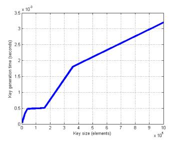
Figure 3. Time to generate chaotic logistic key.
