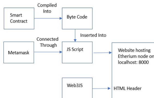
**Figure 1.** Smart contract test bed.
