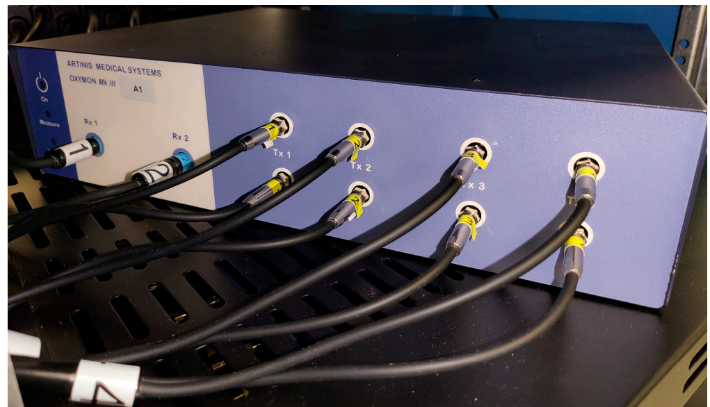
Figure 3. Displaying a portion of the multi-channel OxyMon Mk III device that is used to collect HbO, HHb, tHb, and HbDiff. HbO, oxyhemoglobin; HHb, deoxyhemoglobin, tHb, total hemoglobin; HbDiff, difference between HbO and HHb; NIRS, near-infrared spectroscopy. This figure is from Sainbhi et al. [30], is used under Creative Commons Attribution License (CC BY) [40], and is cropped from the original.
