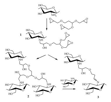
Scheme 3. Mechanism of chitosan cross-linking with TGP.
