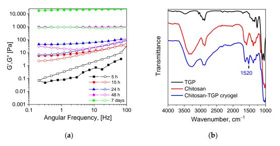
**Figure 1.** Time-dependent mechanical spectra of 3% chitosan solution after addition of equimolar content of TGP at T = 25 °C: filled symbols —storage moduli (G'), open symbols—loss moduli (G'')—(a). FT-IR spectra of TGP, chitosan, and chitosan cryogel cross-linked with TGP at molar ratio TGP:chitosan of 1:4 (b).
