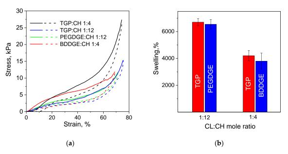
**Figure 2.** Strain–stress curves of the swollen chitosan (CH) cryogels cross-linked with TGP, BDDGE, and PEGDGE at cross-linker (CL):CH molar ratios of 1:4 and 1:12 (**a**). Equilibrium swelling of the cryogels in water (**b**).
