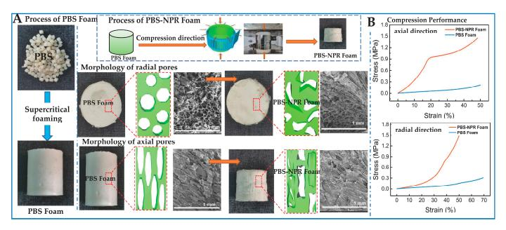
**Figure 5.** The preparation and pore morphology variation after compression direction of PBS-NPR foam and PBS foam (**A**), and the axial and radial compression tress-train curve of PBS-NPR foam and PBS foam (**B**) (Reprinted with permission from ref. [101], Copyright 2021, American Chemical Society).
