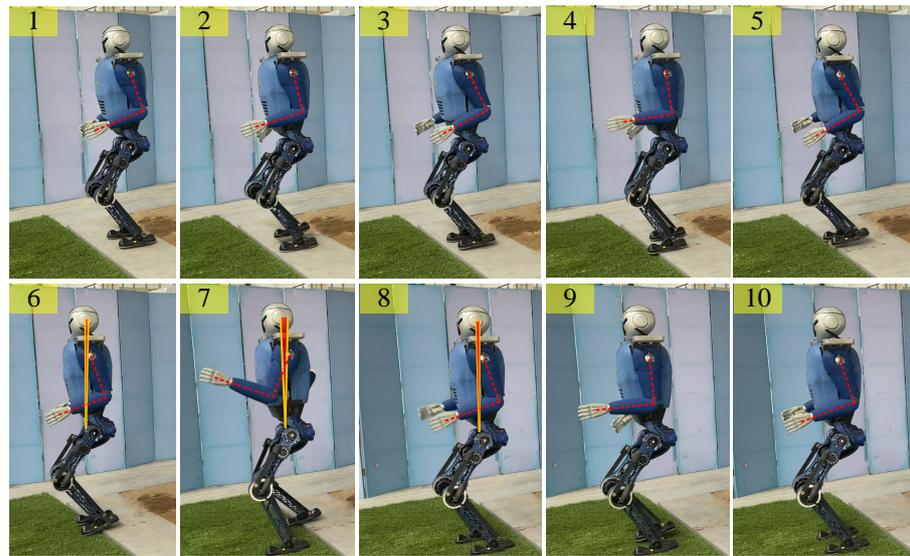
**Figure 5.** Video capture of the momentum compensation recovery of the swing arm when disturbed by the robot’s descending steps. The red fan-shaped area formed between the two yellow lines represents the upper body’s pitch range.
