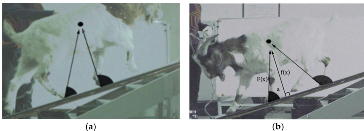
**Figure 2.** Graphical representation of the angle. The black point is the COM, and the included angle is between the propulsive force  $F(x)$  and the upward direction along the slope: (a) uphill; and (b) downhill.
