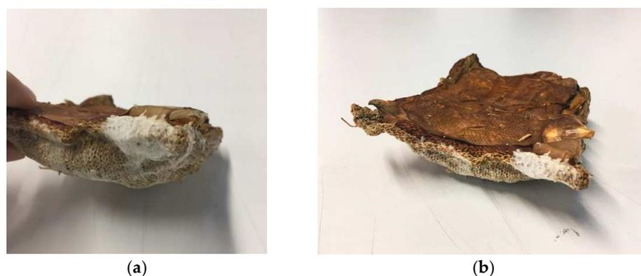
**Figure 9.** (a) Corner of the pocket with white mycelium skin. (b) BC dried onto the pocket, showing pattern of fabric underneath (image credit: authors).
