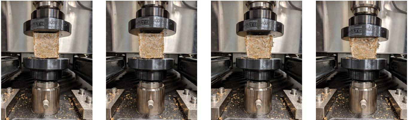
**Figure 3.** Mechanical tests were performed on MBC sample C<sub>33</sub> with a 0.05 mm per second rate with the MTS machine (Figures are taken at 15-s intervals).
