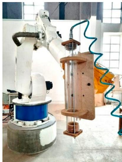
**Figure 8.** The Fabricated Extruder (Image credit: Authors).
