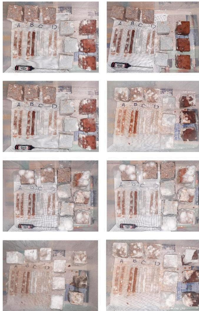
**Figure 6.** Initial material tests for examining treatments' cultivation and gelling agents' performance (Image credit: Authors).
