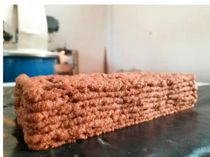
**Figure 10.** The extruded lattice brick (Image credit: Authors).
