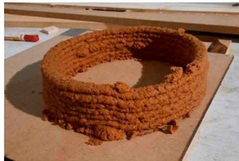
**Figure 9.** The initial extrusion experiment (Image credit: Authors).
