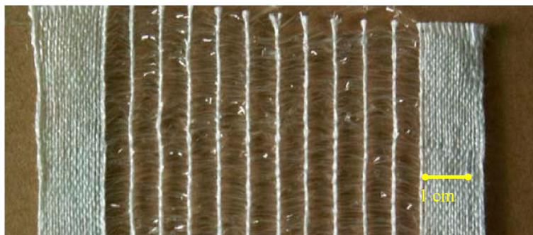
**Figure 7.** Photograph of dry active textile detail. The active bilayer yarn constitutes the clear strips in the weft (horizontal) of the fabric and the white thread is the polyester yarn of the fabric warp (vertical).
