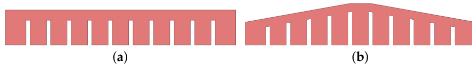
Figure 4. Variation of the shape of the soft bending actuator branches in the gripper: (a) flat, (b) sloped (in the displayed configuration, \alpha is negative).
