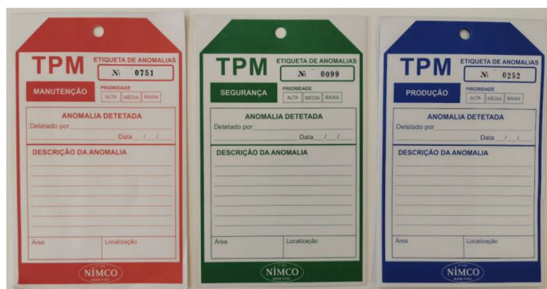
Figure 2. Template of TPM labels for the categories Maintenance, Safety and Production, respectively.
