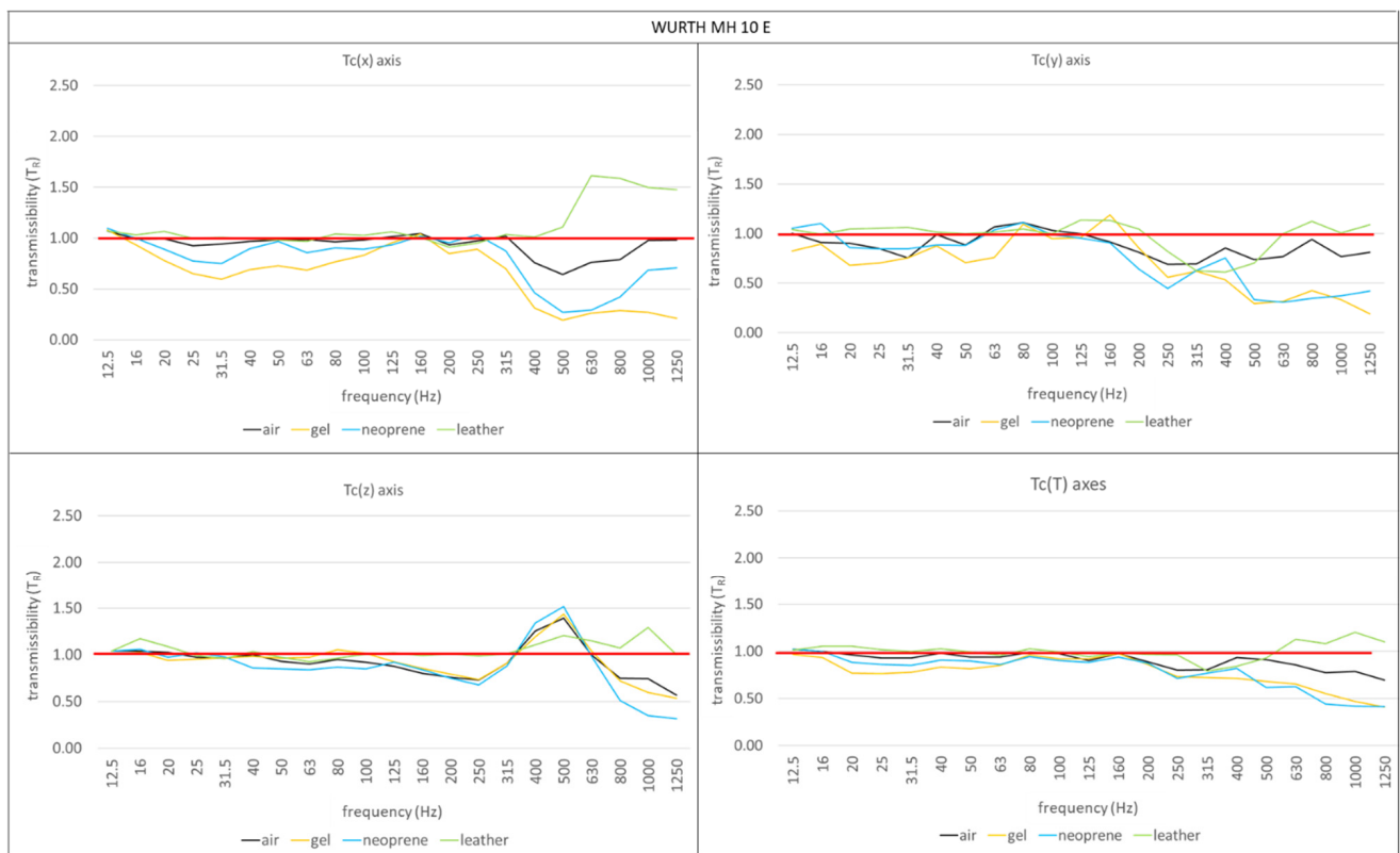
Figure 11. Total triaxial transmissibility, and along every single axis for the hammer Wurth MH 10 E.
