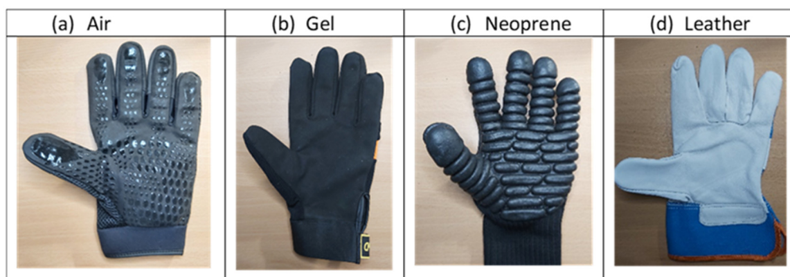
Figure 2. Photos of the tested gloves: (a) glove in air; (b) glove in gel; (c) glove in neoprene; (d) glove in leather.
