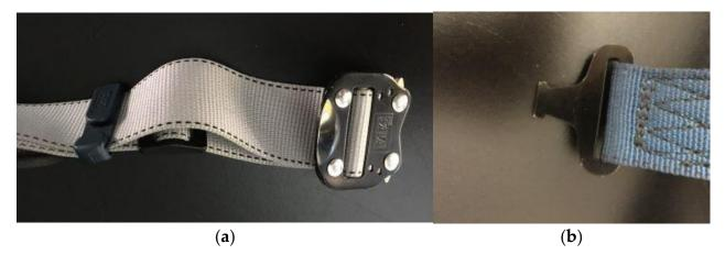
Figure 1. The leg-strap connection: (a) adjustable insertion end and (b) hook end. Photo by Roger Jensen.
