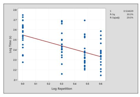
**Figure 5.** Linear regression fit with equation  $\log T = 2.547 - 0.3597 \log R$ .
