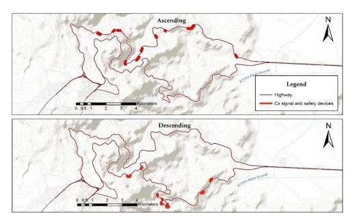
Figure 7. Traffic signals and safety devices condition in mountain zone.
