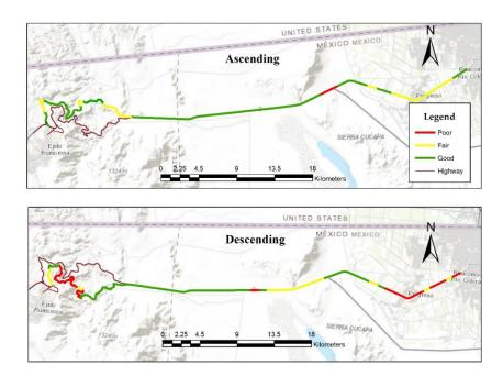
Figure 5. Pavement surface conditions.
