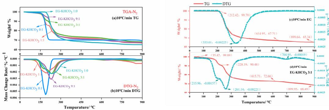
**Figure 2.** TG-DTG curves of five samples placed in a nitrogen atmosphere at a heating rate of 10 °C/min; (a) TG of all samples, (b) DTG of all samples, (c) TG-DTG of EG, and (d) TG–DSC of EG– $\text{KHCO}_3$ .
