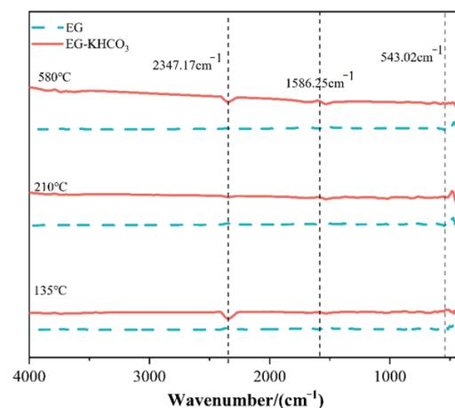
**Figure 4.** Spectra obtained at different temperatures during TG–FTIR analysis.
