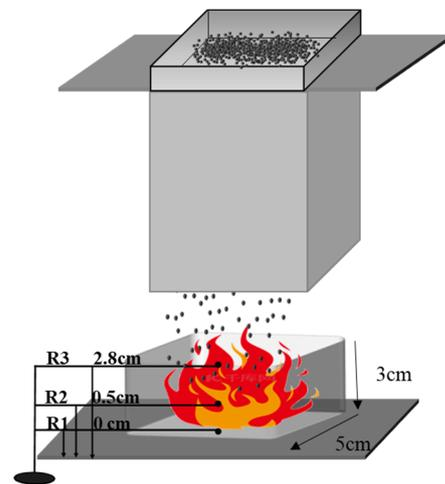
**Figure 1.** Fire-suppression process instrument.
