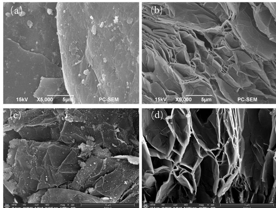
**Figure 7.** SEM images of EG (a,b) and (c,d) EG–KHCO<sub>3</sub> powders.
