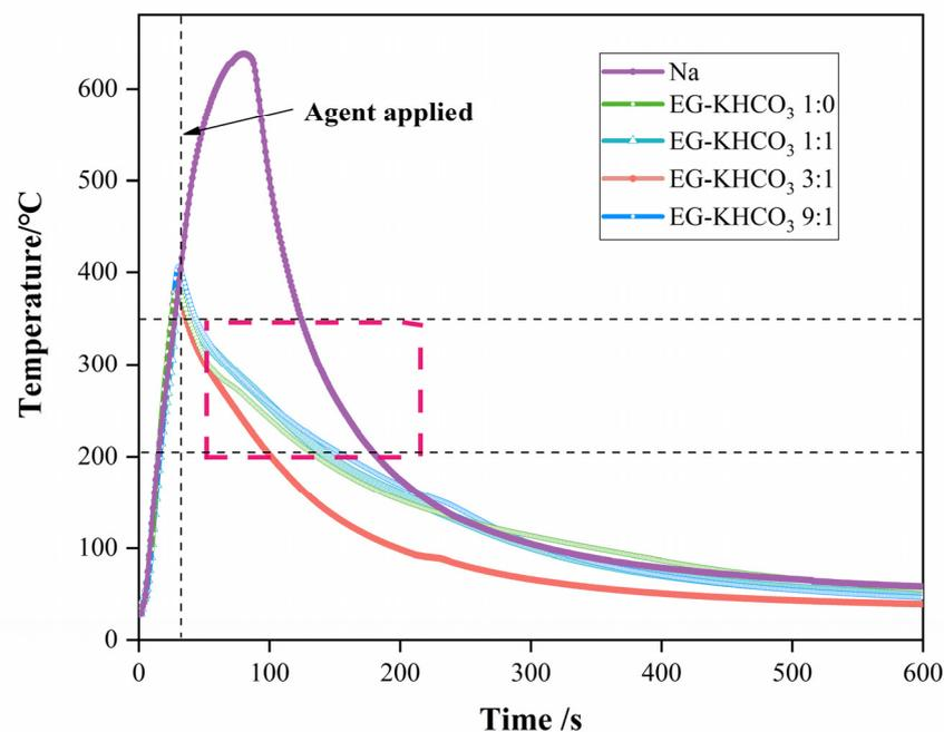
**Figure 8.** Numerical changes measured at thermocouple R1 for the four sample powders during the experiment.
