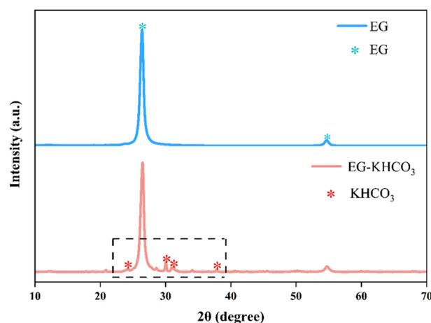
**Figure 6.** XRD pattern of fire extinguishing powder with distinct peaks observed in the dashed line area.
