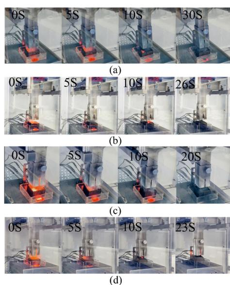
**Figure 3.** Images taken during the fire-extinguishing experiment: (a) EG powder, (b) 1:1, (c) 3:1 and (d) 9:1 EG- $\text{KHCO}_3$  powders.
