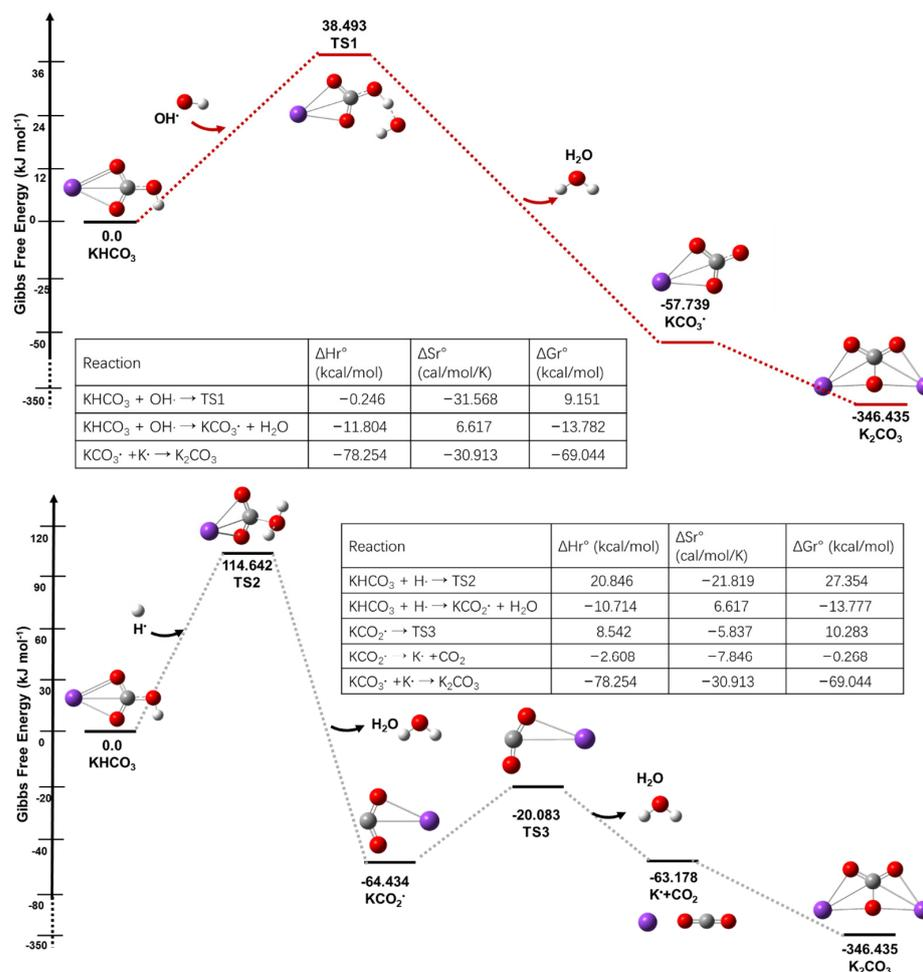
**Figure 5.** Schematic of potential energy of  $\text{KHCO}_3$  reactions (R1, R2). The data along the paths are the relative Gibbs free energy values obtained at the B3LYP/TZVP//CCSD(T)/cc-pVTZ level.
