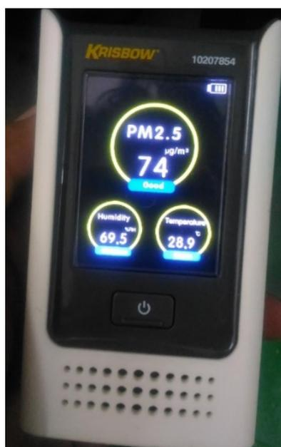
Figure 4. Air quality measuring device.
