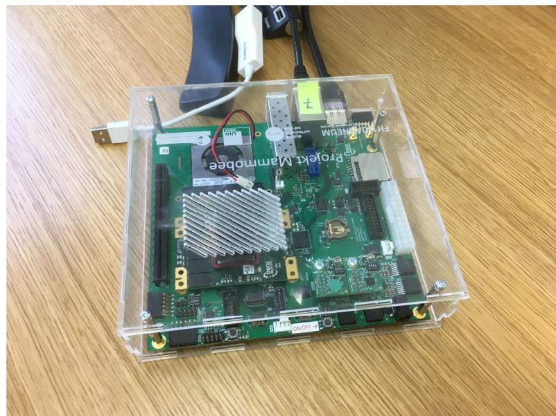
**Figure 6.** Trenc Electronic FPGA hardware enabling ALA parallel computation.
