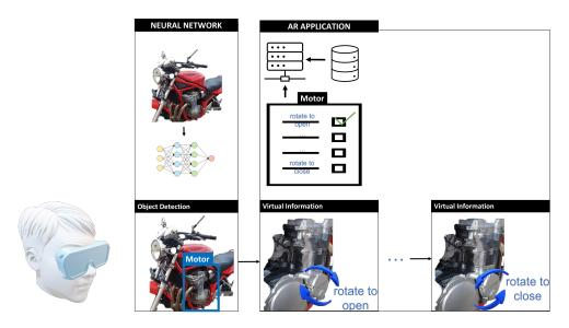
Figure 3. Pipeline of an AR application with a neural network used for object detection.
