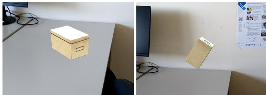
**Figure 7.** Placement of a virtual box onto a surface according to its normal vector. Depending on where the centre of the screen is aimed, the box base is placed parallel to the table (**left**) or to the wall (**right**) and in contact with the surfaces.
