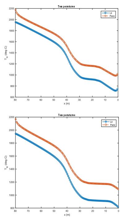
**Figure 4.** Comparison of the temperature profiles obtained with two alternative fuels (above: biomass; below: tires).
