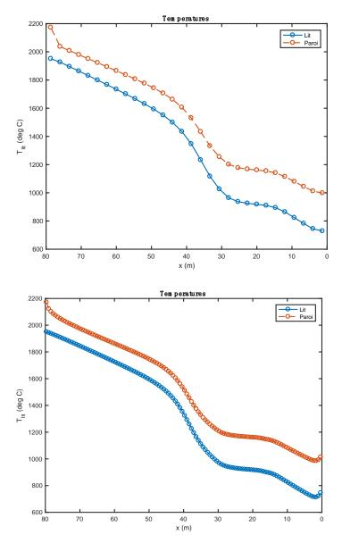
**Figure 6.** Comparison of the temperature profiles obtained with 30 (above) et 120 (below) compute nodes (heavy fuel oil and biomass).
