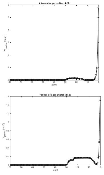
**Figure 3.** Comparison of gas velocity profiles obtained with two alternative fuels (above: biomass; below: tires).
