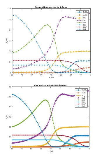
**Figure 7.** Comparison of the meal composition profiles obtained with 30 (above) et 120 (below) compute nodes (heavy fuel oil and biomass).
