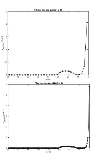
**Figure 8.** Comparison of the gas velocity profiles obtained with 30 (above) et 120 (below) compute nodes (heavy fuel oil and biomass).
