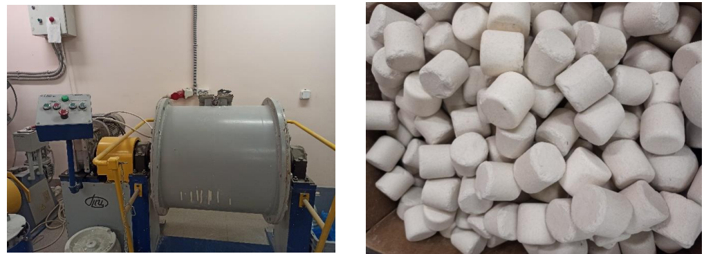
Figure 5. Ball mill and grinding bodies used to grind GBFS.
