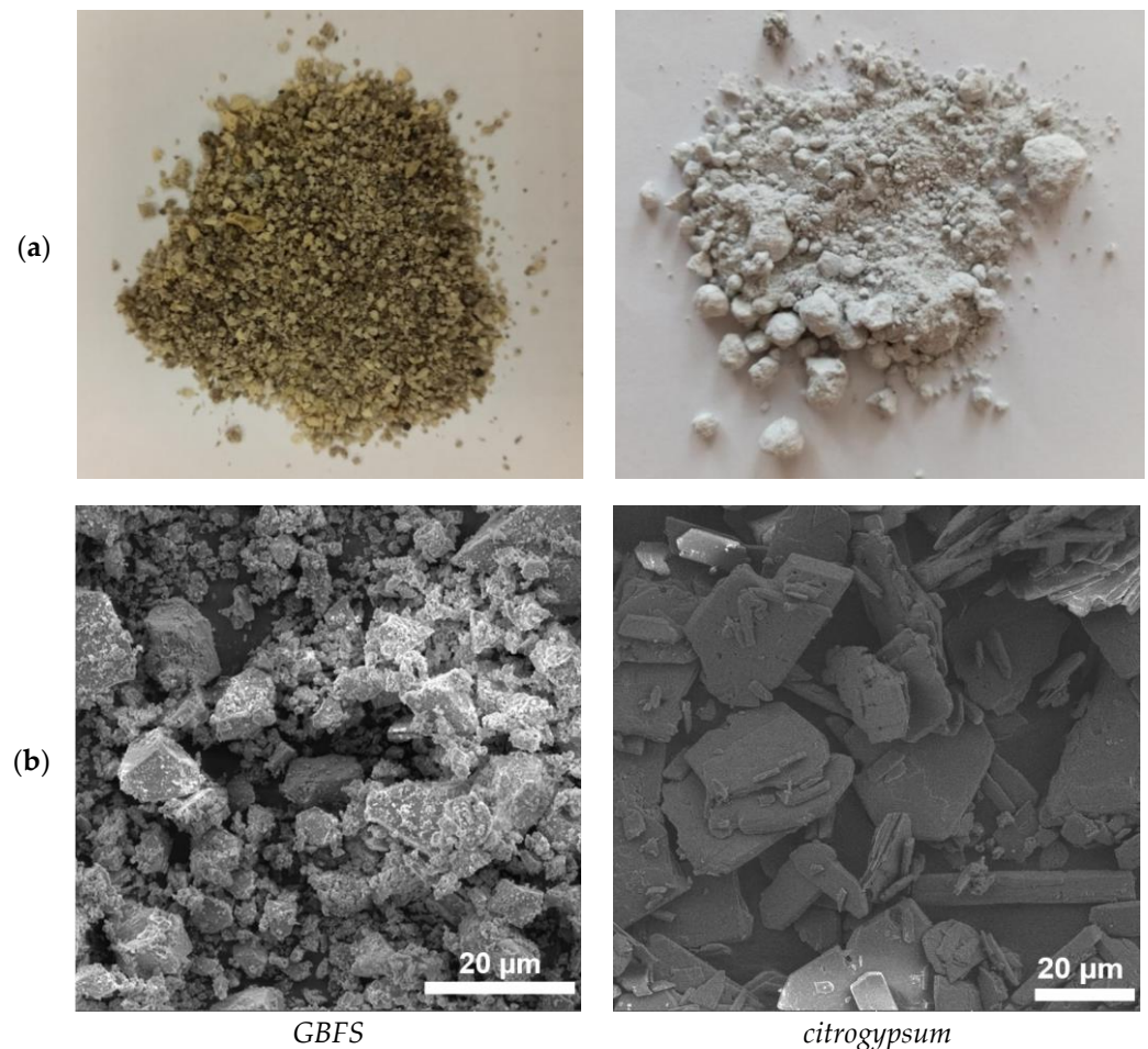
Figure 4. Natural appearance (a) and SEM-images (b) of GBFS and citrogypsum.
