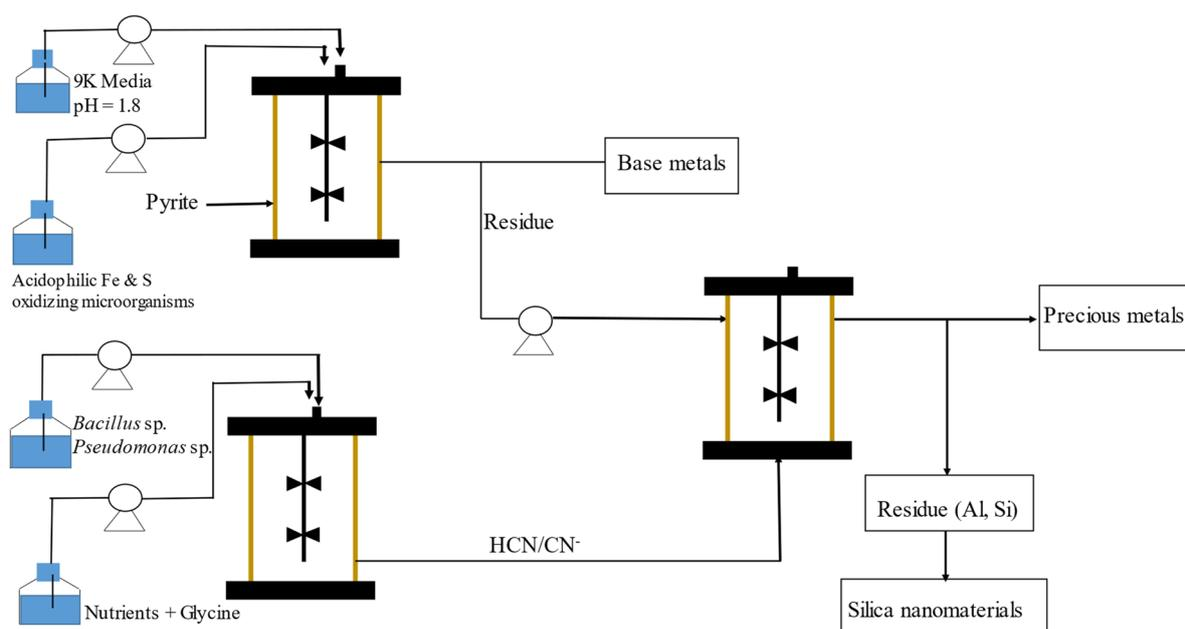
**Figure 2.** Proposed metal extraction process from electronic waste.
