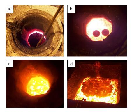
**Figure 5.** Photographs during smelting process in induction furnace: (**a**) loading of BM with scrap (**b**) loading of briquettes on top of melt (**c**) complete melting of scrap and BM (**d**) tapping of alloyed steel.
