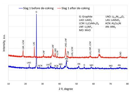
Figure 8. XRD analysis of the first slag before and after de-coking of trial 2 with high-Co BM.
