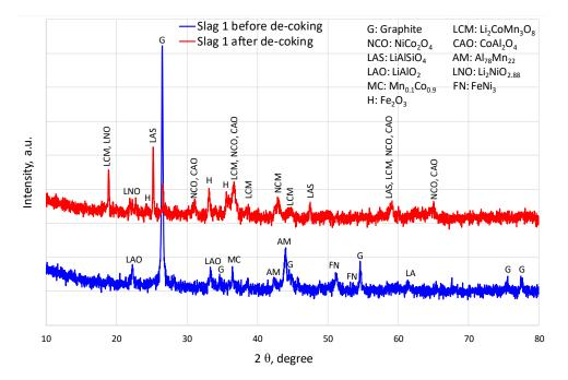
Figure 7. XRD analysis of the first slag before and after de-coking of trial 1 with high-Ni BM.
