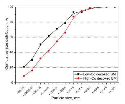
Figure 3. Cumulative size distribution of high-Ni and high-Co BM after de-coking.
