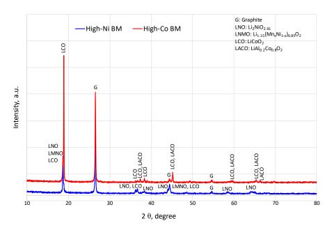
Figure 1. XRD analysis results of high-Ni and high-Co BM.
