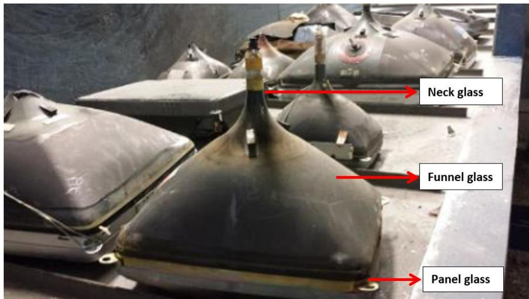
Figure 4. Stripped CRT monitors.
