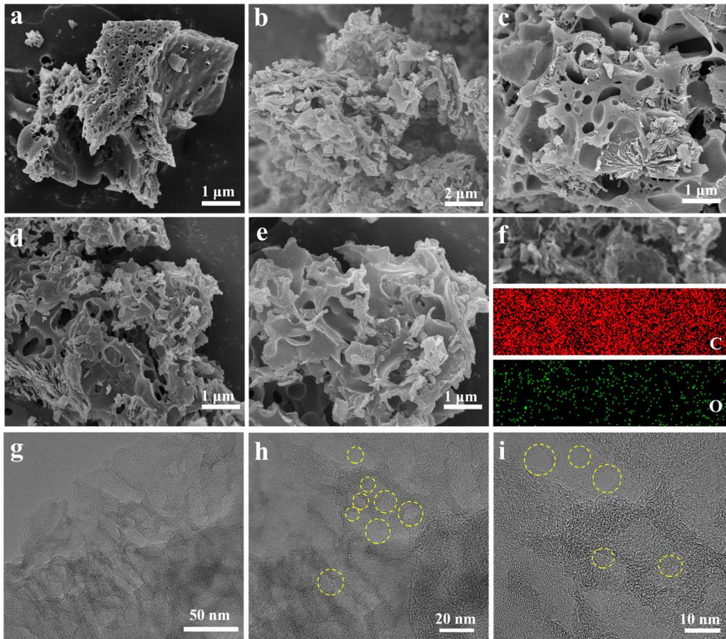
**Figure 1.** SEM images of (a) HPOC-0, (b,c) HPOC-0.5, (d,e) HPOC-1 and (f) Elemental mapping analysis of HPOC-1, (g,h) TEM images and (i) HRTEM images of HPOC-1.
