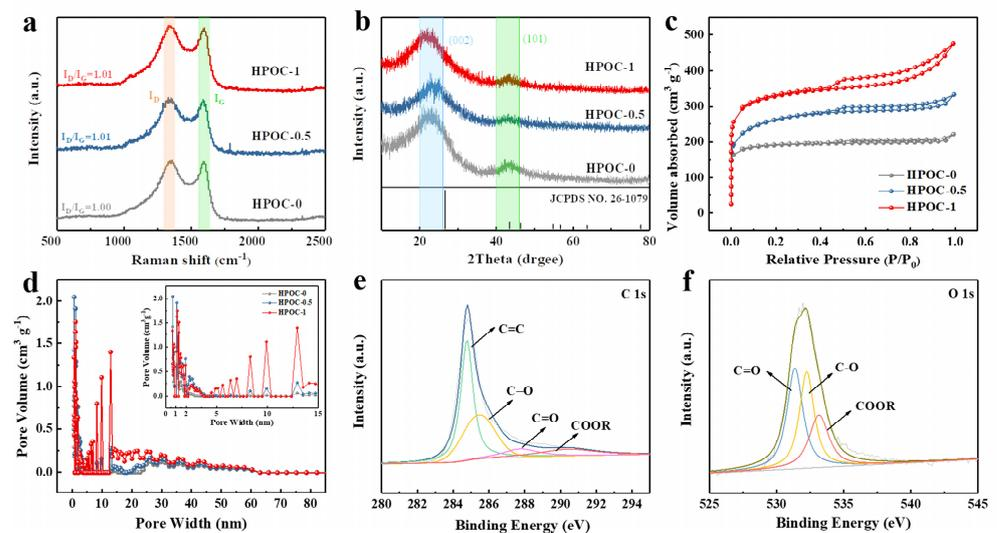
**Figure 2.** (a) Raman spectra, (b) XRD patterns, (c) N<sub>2</sub> absorption/desorption isotherms and (d) pore size distribution curves, (e) C 1s and (f) O 1s spectra of HPOC-1.
