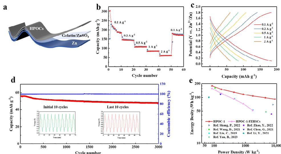
**Figure 6.** Electrochemical performance of the flexible ZHSCs (FZHSCs) device. (a) Schematic of the configuration of FZHSCs device, (b) Rate performance of HPOC-1–FZHSCs at 0.1–2 A g<sup>-1</sup>, (c) corresponding GCD profiles, (d) cycling performance of HPOC-1–FZHSCs at 2 A g<sup>-1</sup> (the inset was the initial and last 10 GCD curves) and (e) ragone plots of HPOC-1-based ZHSCs and reported carbon-based ZHSCs [42,44,51–55].
