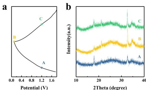
**Figure 5.** (a) Zinc storage mechanisms of Zn//HPOC-1 GCD curve at  $0.1 \text{ A g}^{-1}$  and (b) ex situ XRD of HPOC-1 sample at various states.
