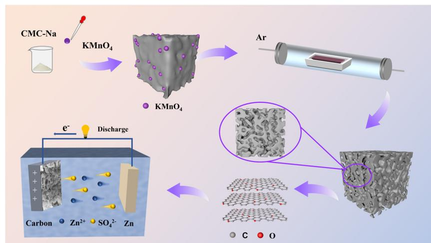
**Scheme 1.** Schematic illustration of the synthesis for HPOCs samples.
