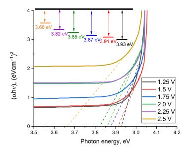
Figure 7. Results of estimation of the band gap of the studied CoZn nanostructures.
