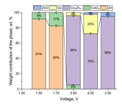
Figure 6. Phase diagram for estimating phase contributions depending on applied potential differences.
