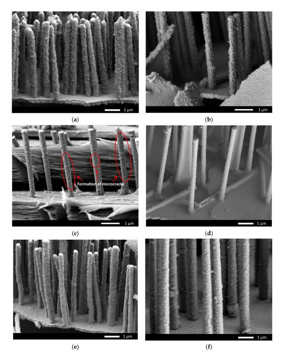
**Figure 11.** SEM images of CoZn nanostructures after life cycle tests: (a) 1.25 V; (b) 1.5 V; (c) 1.75 V; (d) 2.0 V; (e) 2.25 V; (f) 2.5 V.
