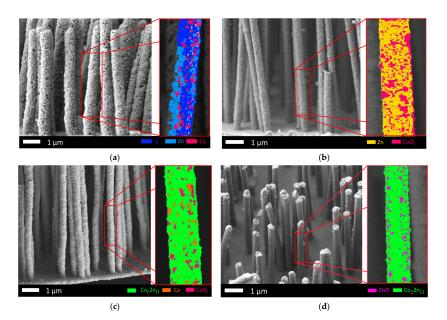
**Figure 5.** Examples of the mapping result of samples with the determination of the phase composition of nanostructures obtained at various applied potential differences, (**a**) potential difference 1.25 V; (**b**) potential difference 1.75 V; (**c**) potential difference 2.0 V; (**d**) potential difference 2.5 V.
