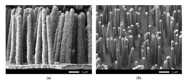
**Figure 2.** Examples of synthesized nanostructures at various potential differences, reflecting the morphological features and the degree of structural ordering of nanostructures: (**a**) nanostructures obtained at a potential difference of 1.25 V; (**b**) nanostructures obtained at a potential difference of 2.5 V.
