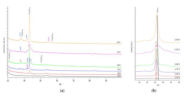
**Figure 3.** Results of X-ray diffraction of the studied samples of nanostructures: (a) X-ray diffraction patterns presented depending on the applied potential difference; (b) Detailed image of diffraction reflections at  $2\theta = 43-43.5^{\circ}$ , reflecting a phase transformation of the Zn  $\rightarrow$  Co<sub>2</sub>Zn<sub>11</sub> type.
