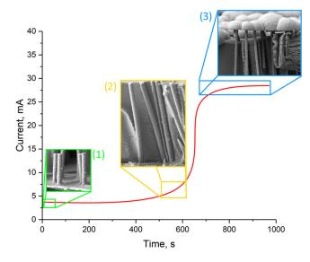
**Figure 1.** Schematic representation of the nanostructures' formation in the pores of polymer matrices using the chronoamperometry method to control the growth of nanostructures: (1) the stage of nucleation of nanostructures; (2) pore filling completion stage; (3) the stage of formation of mushroom-like caps on the surface of polymer matrices, in places of filled pores.
