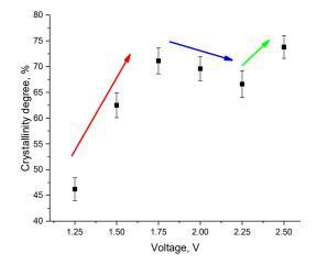
**Figure 4.** Dependence of the change in the degree of structural ordering (degree of crystallinity) on the applied potential difference (The arrows indicate the main stages of the change in the degree of crystallinity: red arrow—increase due to structural ordering during growth; blue arrow—slight decrease as a result of phase transformation processes; green arrow—increase due to the dominance of the  $Co_2Zn_{11}$  phase).
