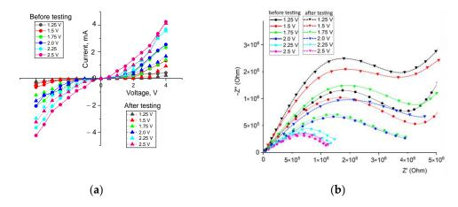
**Figure 10.** (a) IVC curves of CoZn nanostructures before and after life tests; (b) Nyquist plots Z''(Z') before and after life tests (dotted lines with triangles show values afterlife tests).
