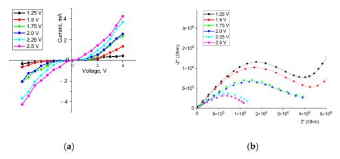
**Figure 8.** (a) Volt-ampere characteristics of the studied CoZn nanostructures obtained under different synthesis conditions; (b) Nyquist plots Z''(Z').
