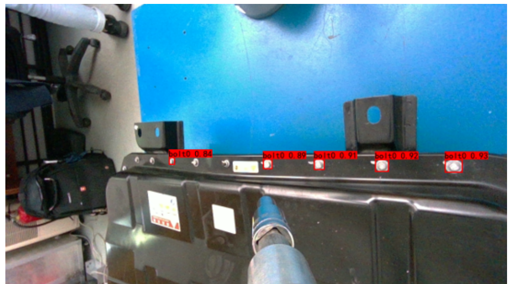
Figure 15. Results of the initial positioning of the screws.
