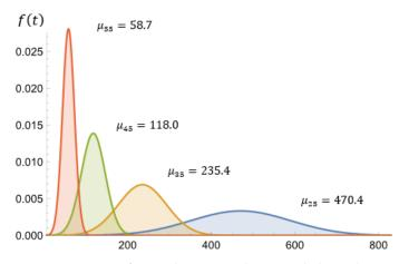
Figure 2. Battery Life Distributions Under Several Thermal Stresses.
