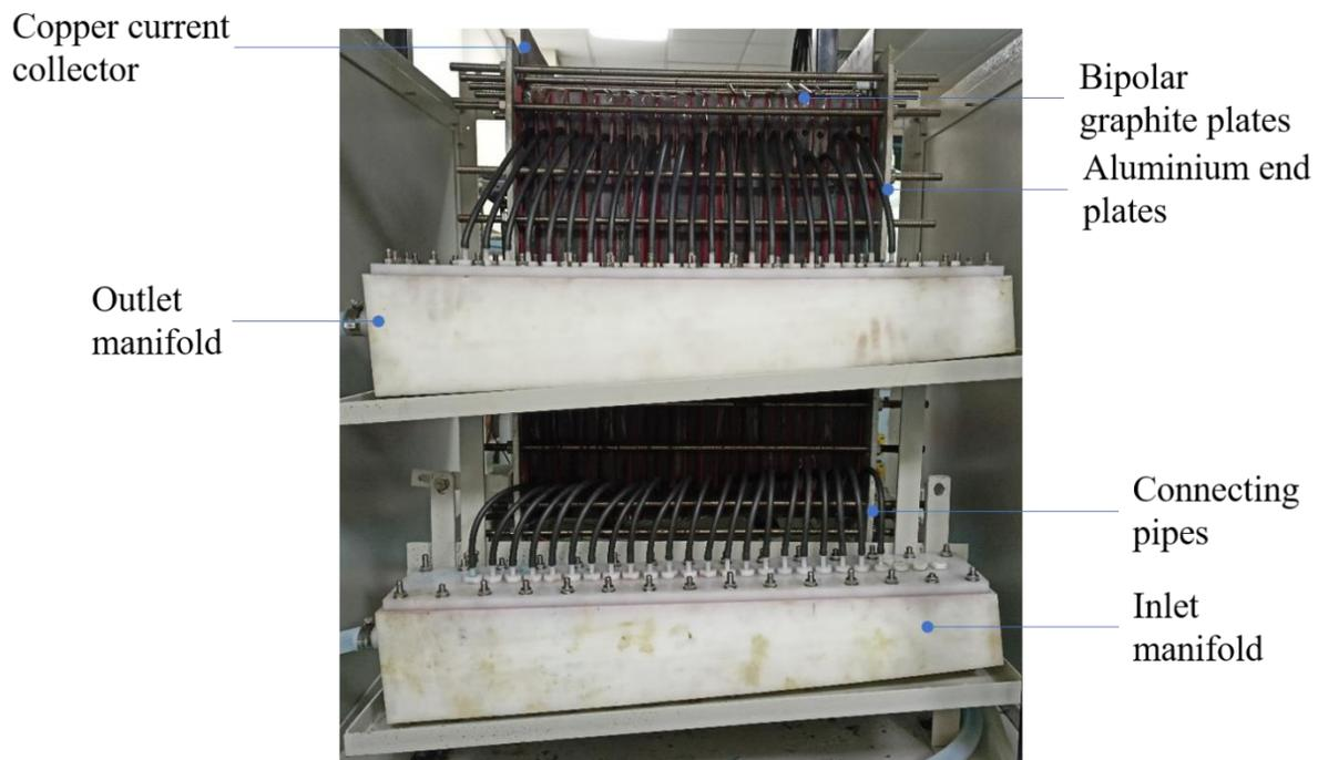
**Figure 1.** The 22-cell VRFB stack with the nominal power of 5 kW and a nominal electrode surface area of 1500 cm<sup>2</sup> that was used for constant power characterization studies.
