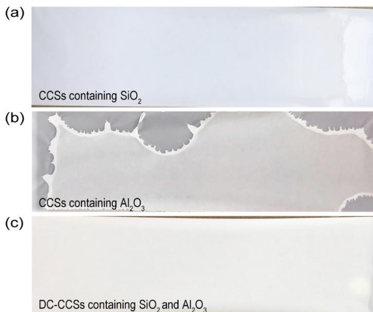
**Figure 3.** Digital camera images of CCSs containing (a)  $\text{SiO}_2$ , (b)  $\text{Al}_2\text{O}_3$ , and (c) DC-CCSs containing  $\text{SiO}_2$  and  $\text{Al}_2\text{O}_3$  (width of separator = 6 cm).
