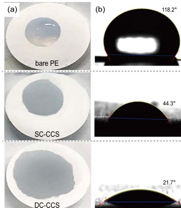
**Figure 5.** (a) Digital camera images of bare PE, SC-CCSs, and DC-CCSs surfaces 5 min after pouring a drop of liquid electrolyte. (b) Contact angle images of bare PE, SC-CCSs, and DC-CCSs surfaces 5 min after pouring a drop of D.I. water (separator radius = 1.6 cm).
