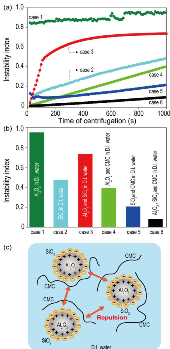
**Figure 1.** Instability indices for various types of aqueous ceramic coating slurries determined using Lumisizer (a) as a function of centrifugation time and (b) at a centrifugation time of 1000 s. (c) A schematic demonstrating the formation of the SiO<sub>2</sub> sheath around the Al<sub>2</sub>O<sub>3</sub> particles, resulting in the stable dispersion of the dual ceramic slurry.
