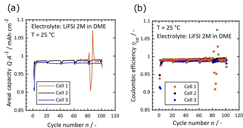
**Figure 3.** Galvanostatic cycling performance of three identical cells with Cu/Li structure. Electrolyte used in all cells is LiFSI 2M in DME. (a) areal capacity and (b) Coulombic efficiency over life time is shown for cells running at  $T_{\text{Cell}} = 25$  °C with the current density of  $J = 1$  mA·cm<sup>-2</sup>.
