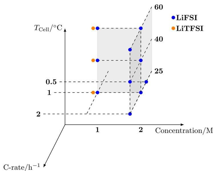
**Figure 2.** Matrix of the conducted measurements. For the salt LiFSI the c-rate was varied with  $I \in \{0.5, 1, 2\}$  C at a salt concentration of  $c = 2$  M and a cell temperature of  $T_{\text{Cell}} = 25$  °C. The temperature was varied with  $T_{\text{Cell}} = \{25, 40, 60\}$  °C at the same concentration and  $I \in \{1, 2\}$  C. At a concentration of  $c = 1$  M measurements at  $I = 1$  C and  $T_{\text{Cell}} = \{25, 40, 60\}$  °C for two salts: LiTFSI and LiFSI.
