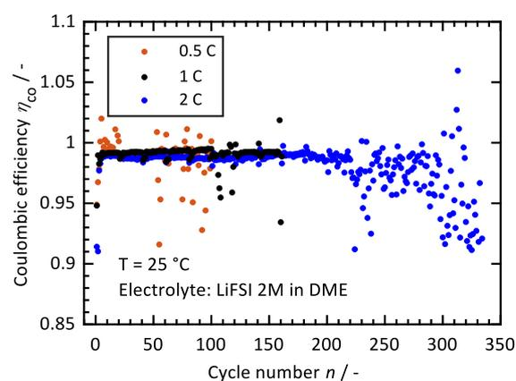
**Figure 4.** Galvanostatic cycling performance of cells with Cu/Li structure using LiFSI 2M in DME as the electrolyte. Cells are run each with an individual C-rate of  $I_{Cell} \in \{0.5, 1, 2\}$  C and are shown with orange, black and blue colors, respectively. The cell temperature for all three experiments was set to  $T_{Cell} = 25$  °C.
