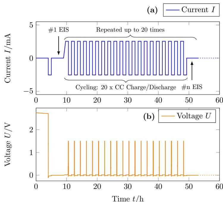
**Figure 1.** Segment of the measurement procedure of the conducted cycling tests example at  $I_{\text{Cell}} = 1 \text{ C}$ . The current data are presented in (a) and the corresponding voltage data are visualized in (b). Before the first cycle and after each 20 full charge/discharge cycles, EIS measurements were conducted.
