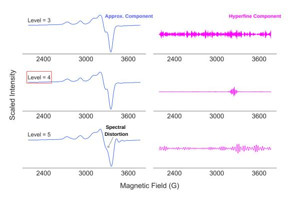
**Figure A1.** WPT analysis of ESR spectra of Cu-AHAHARA complex recorded at 100 K. The approximation and hyperfine components are shown at decomposition levels of 3, 4 and 5 using the Db9 wavelet. In this case, the approximation component at level-5 showed spectral distortion, implying that level-4 is the optimal decomposition level in this case.
