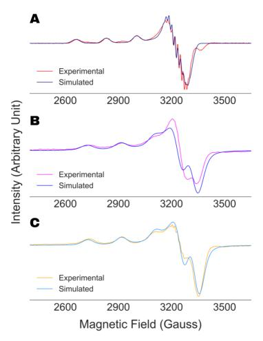
**Figure 6.** EasySpin simulation results along with experimental ESR spectra of SOD1:H48Q (**A**), Cu-AHAHARA spectrum recorded at 10 K (**B**) and 100 K (**C**).
