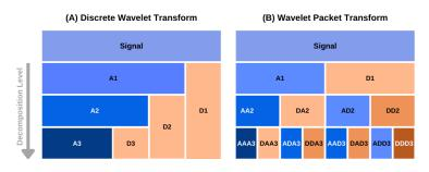
**Figure 1.** A schematic diagram of data decomposition in discrete (**A**) and packet wavelet transform (**B**) methods. The approximation and detail components at level *k* are denoted as  $A_k$  and  $D_k$  in (**A**). In case of wavelet packet transform, the approximation and detail components at a decomposition level are denoted by the component name of the previous level followed by  $A_k$  or  $D_k$ , respectively [27]. Copyright, 2022, The Journal of Physical Chemistry.
