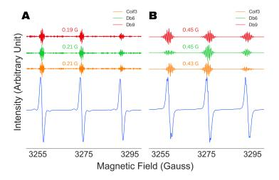
**Figure 5.** Analysis of unresolved and partially resolved X-band cw ESR spectra (blue) of Tempo (**A**) and Tempol (**B**). The superfine spectra recovered by the wavelet packet transform-based analysis of the spectra are shown using three different wavelets, Coiflet-3 (orange), Daubechies-6 (green) and Daubechies-9 (red). Superfine coupling constants obtained are consistent across the analysis involving three different wavelets.
