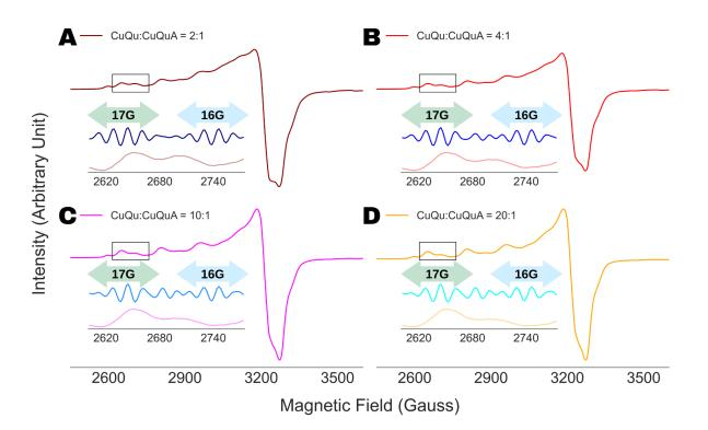
**Figure 3.** WPT analysis of ESR spectra of mixtures of CuQu and CuQuA, mixed in proportions of (**A**) 2:1, (**B**) 4:1, (**C**) 10:1 and (**D**) 20:1, respectively. The insets show the WPT component for the spectral region between 2600 G and 2775 G. Two components were identified in each of the spectral analyses from the difference in nitrogen-hyperfine splitting of 17 G (green double headed arrow) and 16 G (blue double headed arrow).
