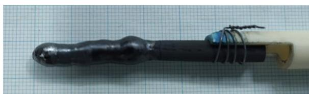
**Figure 2.** A picture of the  $\text{FeCr}_2\text{O}_4$  crystal grown by the optical floating zone method (see text).
