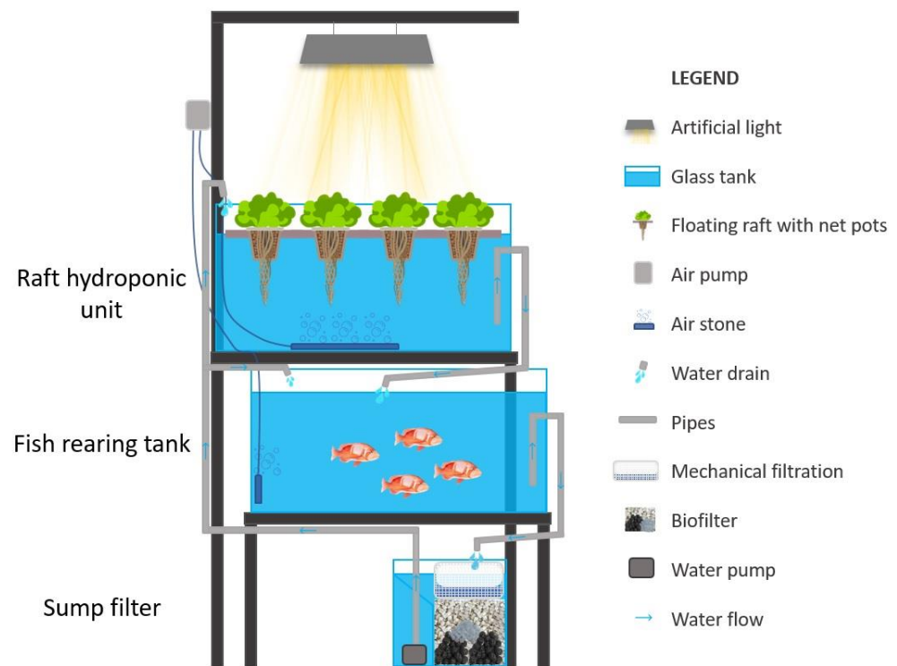
Figure 1. Schematic side view of an autonomous aquaponic system.
