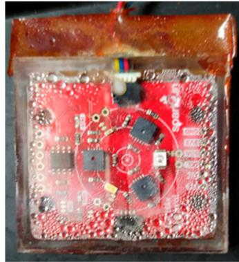
**Figure 13.** Leaking sensor box, two days after the completion of the experiment.
