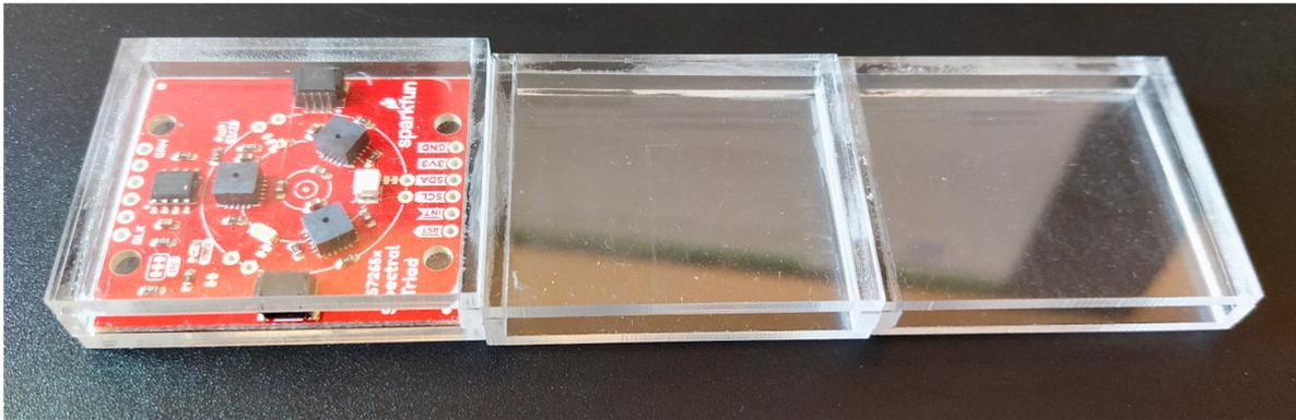
**Figure 1.** Unsealed acrylic boxes used for determining thickness. From left to right: 3 mm, 2.5 mm, and 2 mm. The same sensor was placed in each box and tested.
