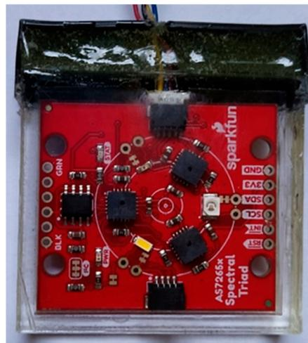
**Figure 2.** AS7265x waterproofed in 2 mm case, sealed with acrylic adhesive and epoxy resin.
