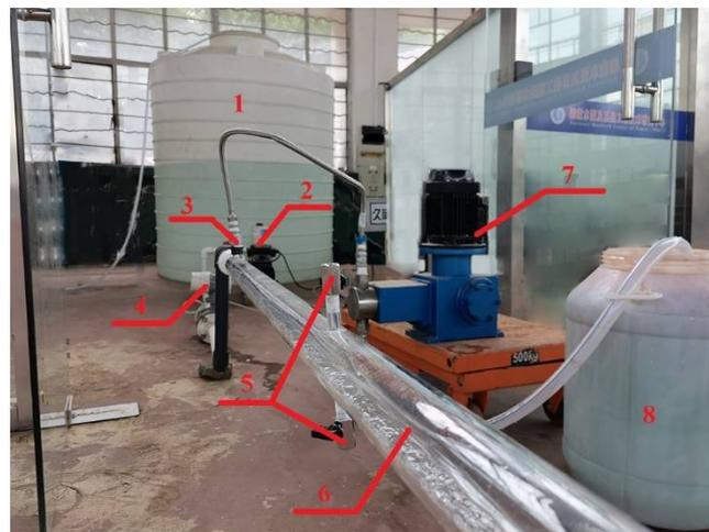
**Figure 1.** Experimental equipment site. (1) Water tank, (2) Centrifugal pump, (3) Fertilizer injection pipe, (4) Flowmeter, (5) Sampling point, (6) PE transparent pipe, (7) Plunger pump, and (8) Fertilizer tank.
