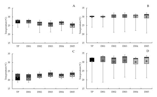
DH5) increased the efficiency of maintaining cool temperature more than using thermal insulation materials without room cooling (DH2 and DH3).
